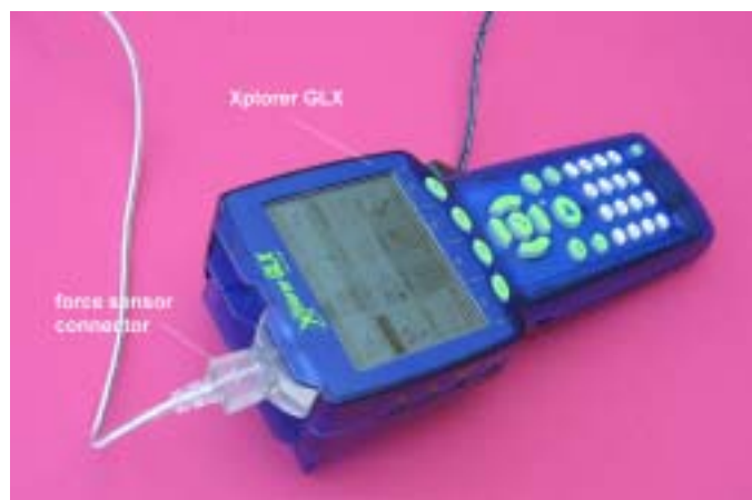
Figure 10 Force sensor plugged into the GLX
