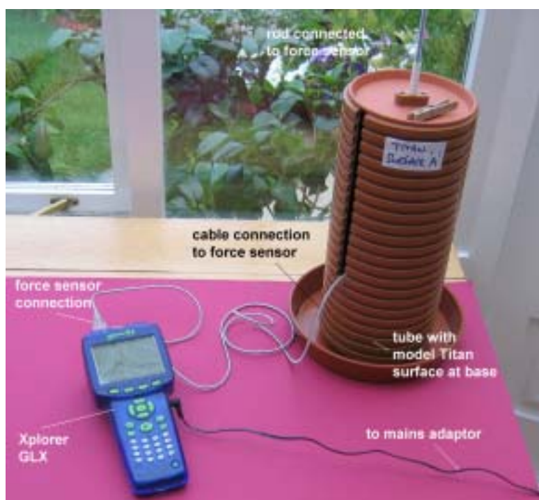
Figure 7 Setup of Xplorer GLX with Huygens Titan lander
