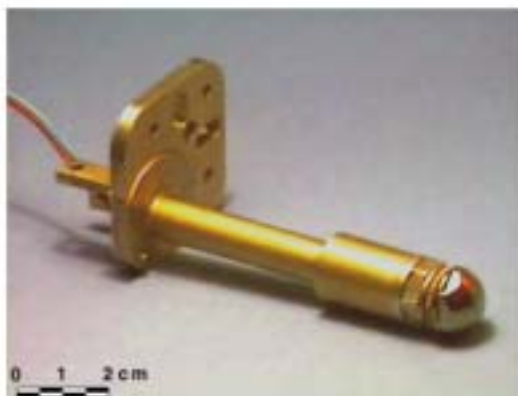
Figure 5 Force sensor ACC-E on the Huygens probe (Courtesy Planetary and Space Sciences Research Institute, The Open University)
